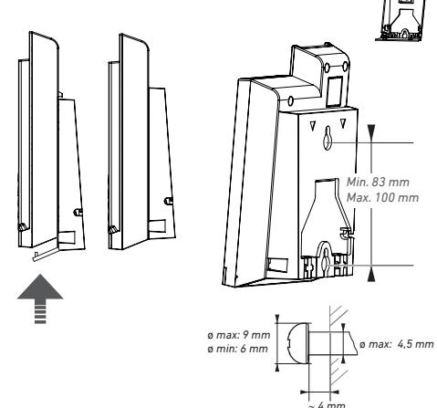
**C Connecting · Anschließen · Connecter · Conectar · Collegare**
